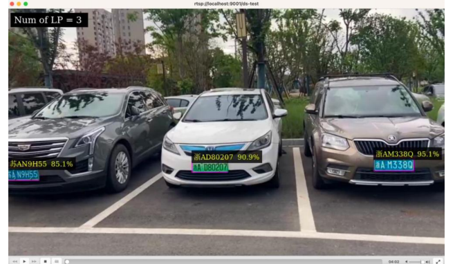
Fig 4. DeepStream output of the proposed LPR pipeline on a parking-lot scene
