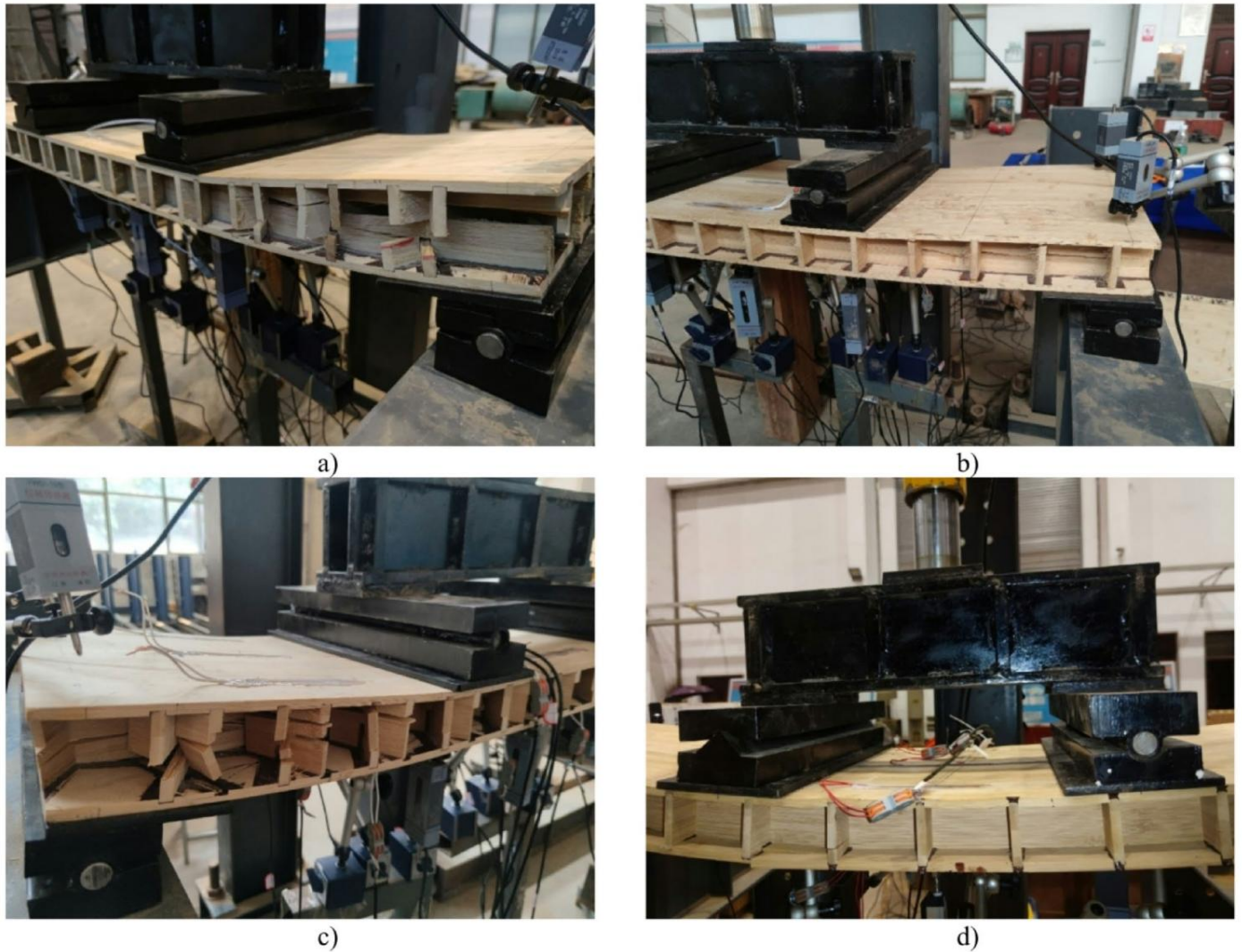
Fig 11. Failure modes of BSP under bending loads (a) BSP-TI (b) BSP-SI (c) BSP-KI (d) BSP-SP
