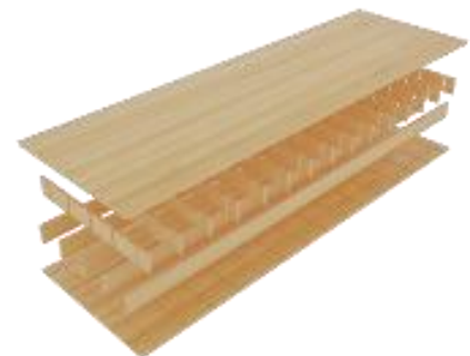
Fig 4. Schematic diagram of laminated bamboo square lattice sandwich panel processing by partition method
