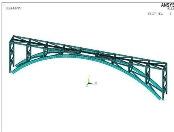
Fig 2. FE model of the glulam arch bridge
