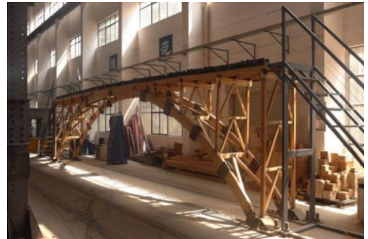
Fig 1. Structural model of the glulam arch bridge
