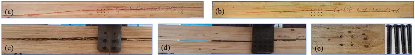
Fig 6. The splitting failure modes of the first group: (a) crack along the wood grain direction, (b) limited-length crack, (c) fiber bridging, (d) no fiber bridging and (e) undistorted bolt hole and bolt
